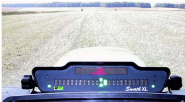
User interface of tracking system. Diodes show actions that the driver should take.
