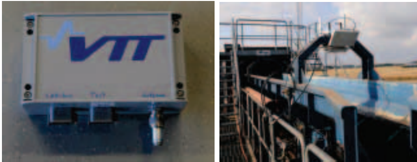
Figure 4.9-3: Developed RFID reader for the harvester and a test reader set-up at a saw mill.
