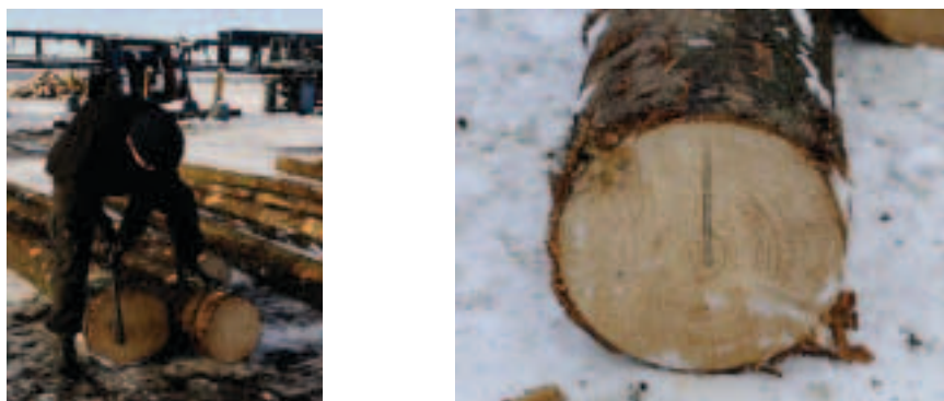
Figure 4.9-2: Manual application of the transponder into the log end.
