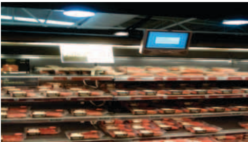
Figure 4.4-3: Electronic display above RFID-enabled fridge shelves.
