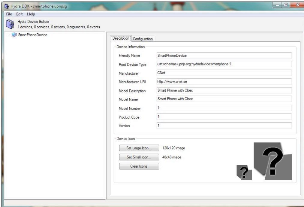
Then one adds the service created in the previous section by right clicking on the device in the left pane.
