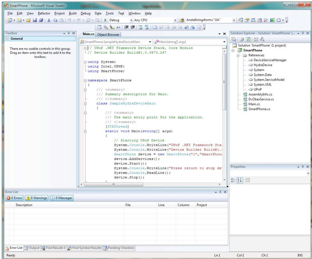
The device code is already runnable since all methods are stubbed. Normally one would then change the code in the stubs to do the actual device communication. The location of the stubs to be changed is in "Device name".cs, i.e. `SmartPhone.cs` in this project. But in this case we will start the device by opening the "Debug" menu and selecting "Start debugging".
