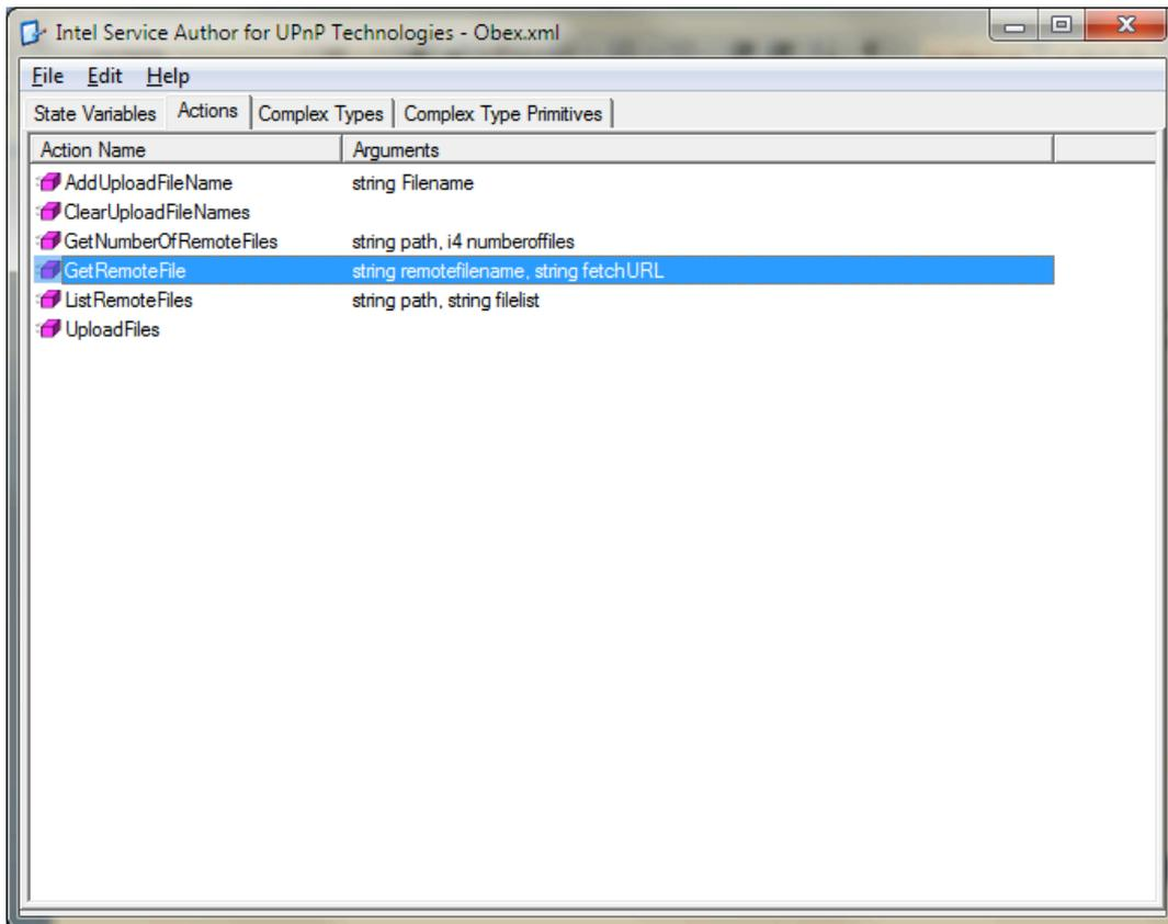
Here we have defined a number of methods with their corresponding arguments. The methods are added using the "Action Editor" which allows for adding arguments and defining in which direction it is used, see below.
