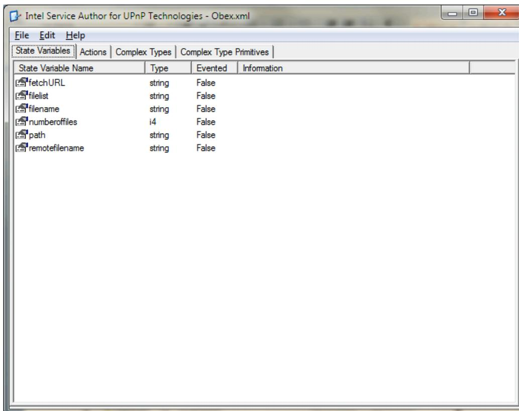
The first step is to define the state variables that will be used by the service. State variables have to be defined for all Input/output parameters used in the service. In this case we have a number of state variables defined with their respective types.
