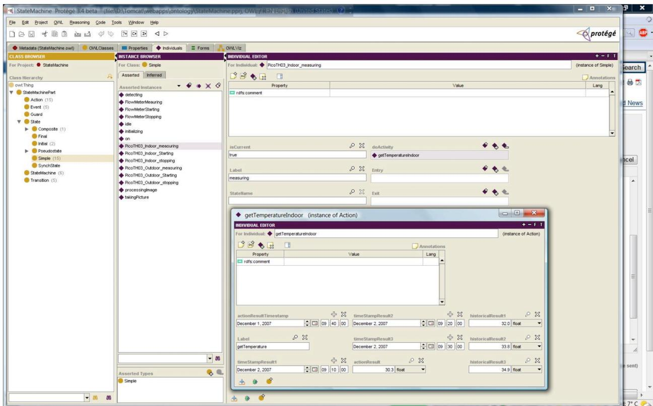
2. Add the "doActivity" associated with a state by clicking on the button 'create new resource' followed the "doActivity" property. For the measuring state, this is the "getTemperatureIndoor" activity, which is used to model the indoor temperature measuring. An instance of data (not mandatory) is shown in above figure.
